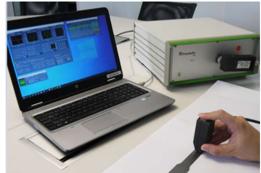
Figure 1: 3MA system applied to a lab sample
