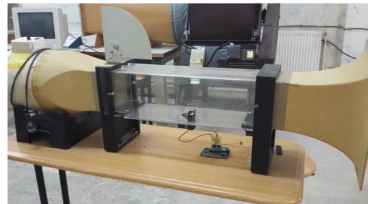
Figure.7. The anemometer probe in the wind tunnel.
