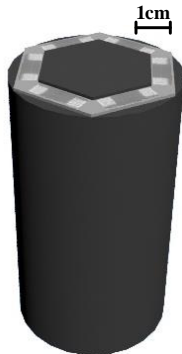
Figure.5. The probe embedded with the hexagonal MEMS hot-film sensor chip in its cavity.
