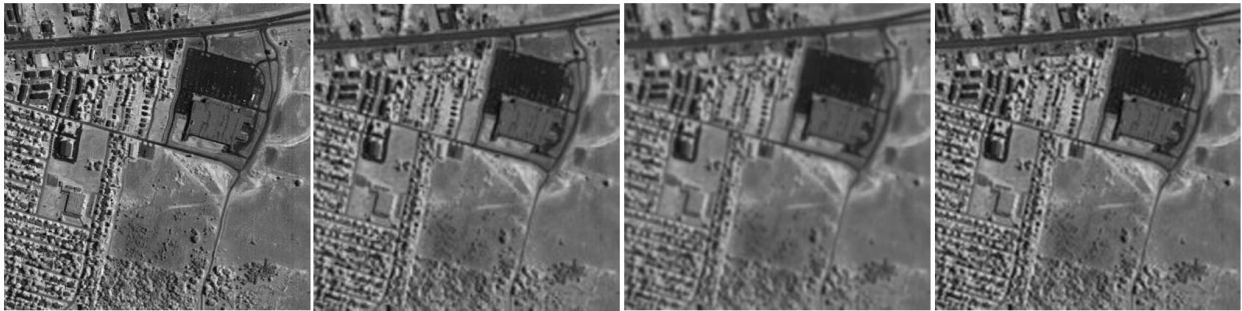
Fig.7. From left to right: a) The original “Urban” image from AVIRIS, b) Bicubic Interpolation, c) Spline Interpolation and d) WSRnet algorithm (all with an upscaling factor of x2)
