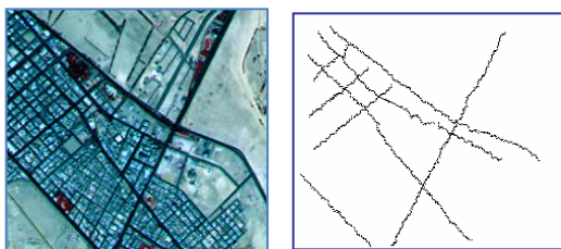
Fig 3 →(a) Original image Riyadh SPOT4 10m resolution, (b) road network extracted.
